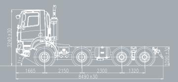
Other possible standard wheelbase: axle 2-3: 2,560/2,950/3,360mi axle 3-4: 1,450mm
