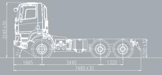
Other possible standard wheelbase: axle 1-2: 3,900/4,500 mm axle 2-3: 1,450 mm
